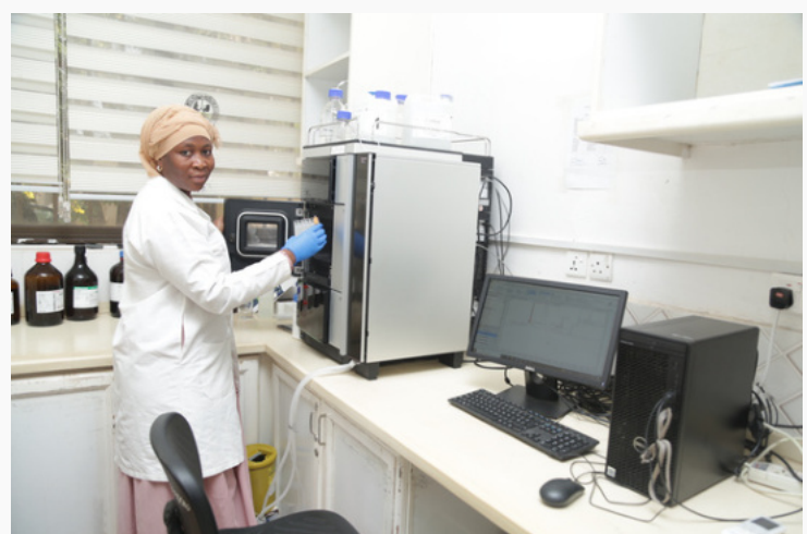
Figure 8: Vitamin A and Haemoglobin variant analysis using HPLC and DAD and autosampler
